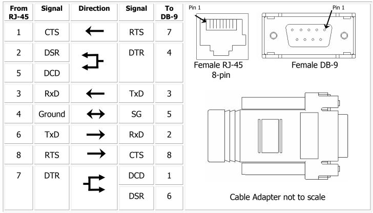
\* Arrows indicate which direction the signal is flowing
