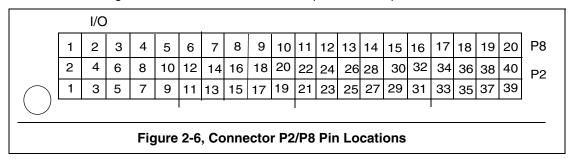
The definition of P2, which has I/O signal interface is shown below.
