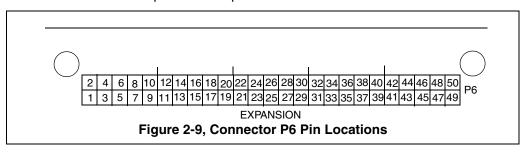
The definition of P6, which has the memory interface signals, is shown below.
