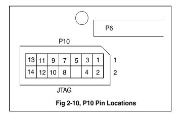
The definition of P10, which has the JTAG signals is shown below...
