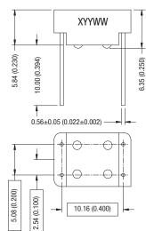
Unless otherwise stated all dimensions in mm (inches)  $\pm 0.25$  (0.01). All pins on a 2.54 (0.1) pitch and within  $\pm 0.25$  (0.01) of true position. Package Weight: 1.1g Typ.
