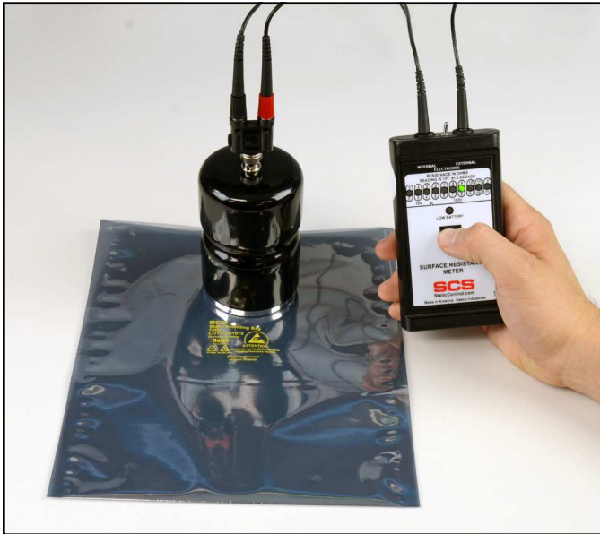
Figure 3. Using the Concentric Ring Probe with the SCS SRMETER2 Surface Resistance Meter
