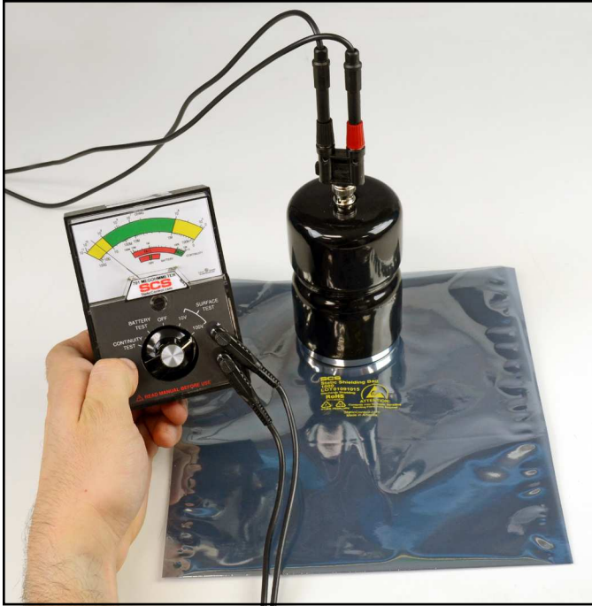
Figure 2. Using the Concentric Ring Probe with the SCS 701 Analog Surface Resistance Megohmmeter
