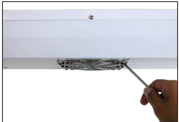
Figure 8. Shorting the ionizer’s two fan grills
