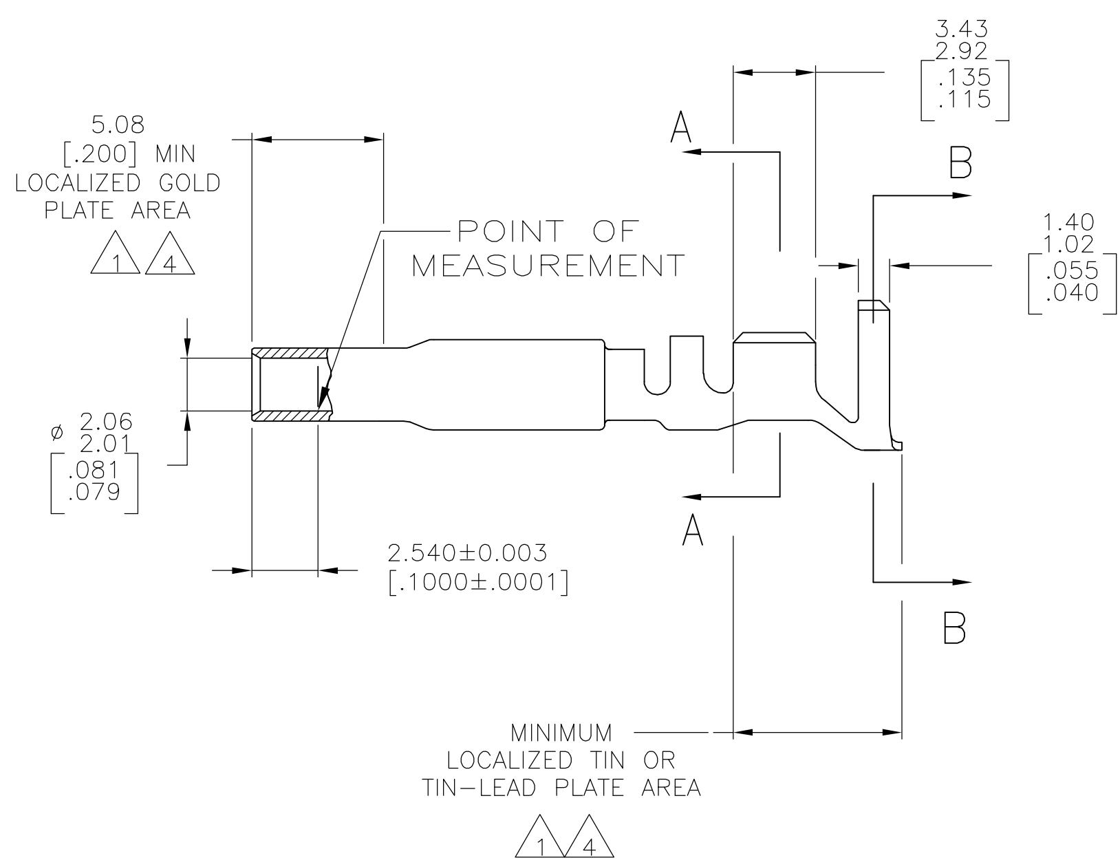
1. 0.00076[.000030] MIN GOLD AT POINT OF MEASUREMENT IN THE LOCALIZED GOLD PLATE AREA, 0.00127[.000050] MIN TIN-LEAD IN TIN-LEAD PLATE AREA, 0.00127[.000050] MIN NICKEL UNDERPLATE ON ENTIRE CONTACT.
