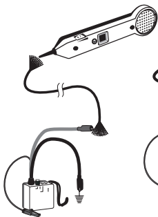
Figure 4a. Cable Tracing
