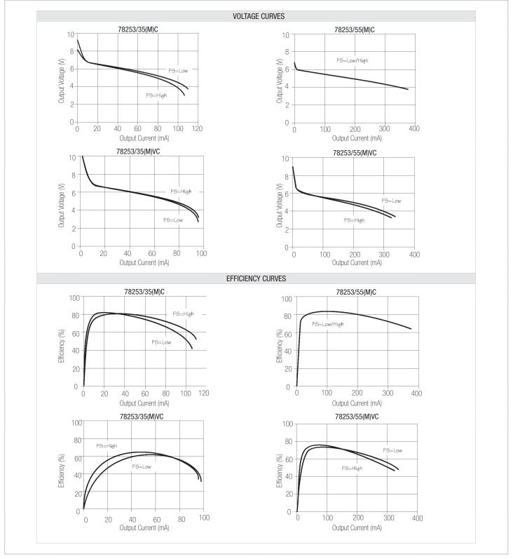
All curves are derived from testing with the Maxim MAX235 IC using the circuit shown in application note MPAN-03 (download at http://www.murata-ps.com/data/apnotes/mpan-03.pdf).
