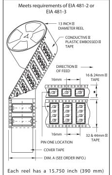
\* Insert "R" before the "T" in the Grayhill part number for tape and reel packaging (500 switches/reel). \*\* Note: 100% matte tin terminal plating does not meet MIL-S-83504 for lead content.
