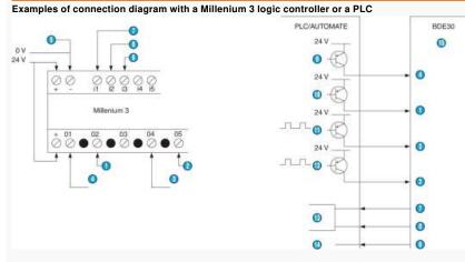
NB : The "tachometer" and "actual direction of rotation" card outputs must be connected to inputs i1 and i2 respectively in order to be able to use the Motomate high-speed counter function.
