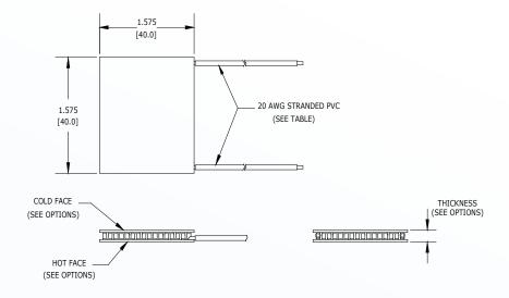
Ceramic Material 96% Alumina Ceramics Solder Construction: 138°C BiSn
