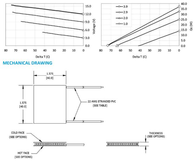
Ceramic Material 96% Alumina Ceramics Solder Construction: 138°C BiSn
