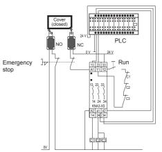
The KNA3-XS interrupts the 24 V supply to the PLC outputs (33-34)
