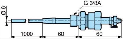
Electrode holder with a single probe supplied in a standard length of 1000mm. (304 stainless steel). Mounting with external 3/8" BSP thread and hexagonal head. Use 24 mm. spanner for hexagon. Suitable for use on boilers, autoclaves and under high temperature conditions up to 200 °C and high pressure conditions up to 25 kg/cm 2
