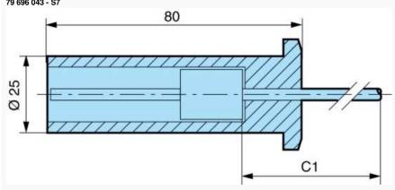
Protected electrode for mounting by suspension. Protective shell : PUC (S7) Electrode : stainless steel. Length of cable as requested (C1) : 79 696 001
