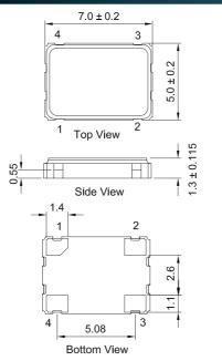
PAD FUNCTION: 1: ENABLE CONTROL 2: GND 3: OUT 4: VDD
