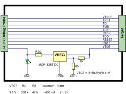
3.6 V 3.3 V 2.5 V 1.8 V 1.0 V 360 k 47 k 330 k 47 k 240 k 47 k 160 k 47 k 68 k 47 k ~400 mA ~400 mA ~300 mA ~200 mA ~150 mA (1, 2) (1, 2) (3) (3) (3)
