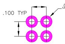
.080 DIA PAD COMP & SOLDER SIDE .042 DIA HOLE PLATED THRU
