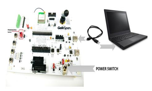
**Step 3**Open the GainSpan Serial Flash Programmer GUI application and select Serial-to-WiFi firmware using the UART interface from location <EVK PACKAGE>\Tools\GS\_programming\_tool\gs2k\_flashprogram.exe Program the EVB.
