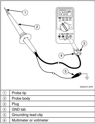
Figure 1. 80K-15 Electronic Air Cleaner Probe
