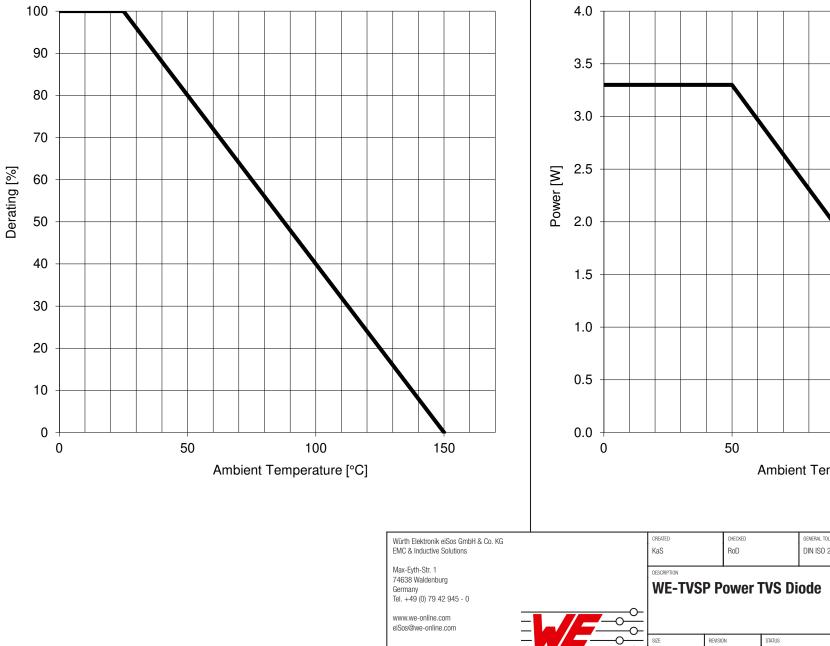
**Steady State Power Dissipation Derating**
