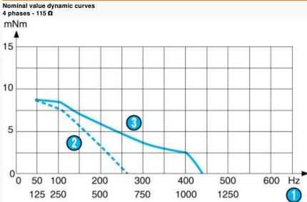
Measurement conditions : 89990101 constant voltage supply board, 17 V at motor terminals, 2 phases energised, full steps, inertia of measuring system 4.53 g.cm2
