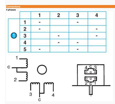
Energisation sequence for clockwise rotation : 2 phases energised (viewed from shaft end, front forward) Commons connected to positive.
