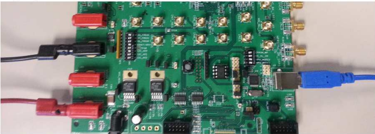
Figure 2. Connecting the Board to the Power Supply and USB Port
