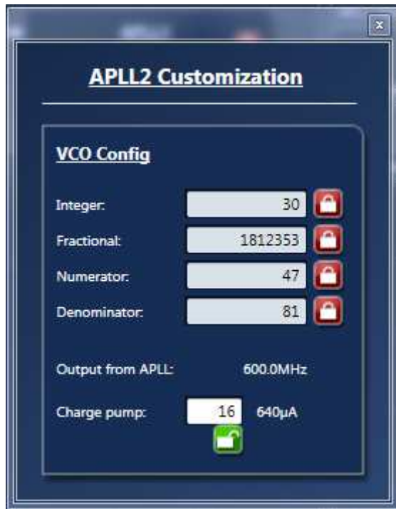
Figure 14. Configure APLL2 Parameters for VCO = 600.0MHz
