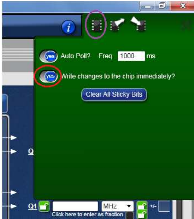
Figure 19. By default, any modifications to the existing configuration data will be written to the device registers immediately
