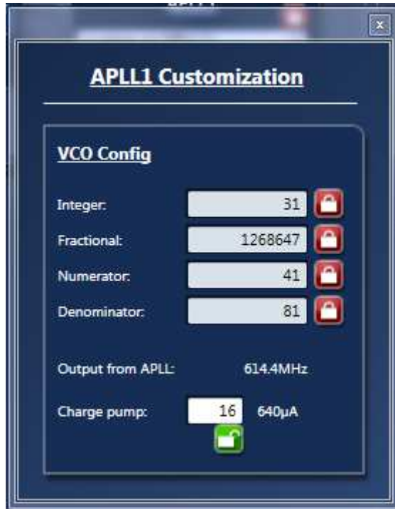
Figure 13. APLL1 Parameters for VCO = 614.4MHz
