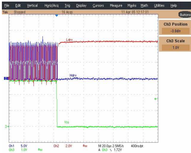
Figure 8 - Shutdown by shorting the SS pin Ch1: Hdrv, Ch2:Ldrv,, Ch3:SS I_{Load}=5A
