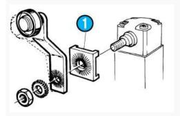
Lever settings or positions dictated by direction in which block 1 is fitted
