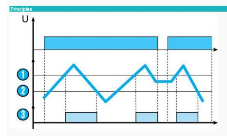
Monitoring two levels, emptying function (level : 2, function Dwn LS (Low Sensitivity :  $250 \Omega$  to  $5 k\Omega$ ), Dwn St (Standard Sensitivity :  $5 k\Omega$  to  $100 k\Omega$ ), Dwn HS (High Sensitivity :  $50 k\Omega$  to  $1 M\Omega$ ).
