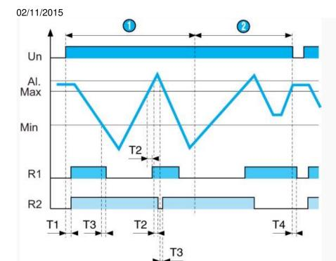
On power-up, probes Min, Max are submerged and probe AI. is above the level of the liquid. Relays R1 and R2 are energised and the pump is ON : emptying starts, the LED for relay R1 is lit. When the Min probe emerges, relay R1 de-energises and the pump if OFF : emptying stops, the LED for relay R1 goes off. If, in the event of a fault, the level continues to rise a nd reaches proble AI., relay R2 de-energises and the alarm is triggered : the LED for relay R2 is lit. This fault can be stored.
