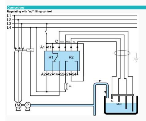
Note : In case of metalic tank, it could be used as probe (C). A green LED indicates the presence of the supply voltage A yellow LED indicates the satus of the output relay A red LED indicates the status of the alarm
