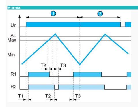
On power-up, the level in the tank is low, relays R1 and R2 are energised and the pump is ON : filling starts, the LED for relay R1 is lit. When the level reaches the Max probe, relay R1 de-energises and the pump is OFF : filling stops, the relay LED goes off. If, in the event of a fault, the level continues to rise and reaches proble Al., relay R2 de-energises and the alarme is triggered : the LED for relay R2 is lit. This fault can be stored.
