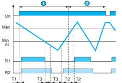
On power-up, probes Min, Max and AI. are submerged, relays R1 and R2 are energised and the pump is ON : emptying starts, the LED for relay R1 is lit. When the Min probe emerges, relay R1 goes off. If, in the event of a fault, the level continues to fall and probe AI. emerges, relay R2 deenergises and the alarm is triggered : the LED relay R2 is lit. This fault can be stored.
