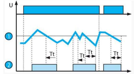
**One-level control (min. probe), emptying function, off-delay** (Level : 1 - off-delay, LS emptying function (Low sensitivity : 250Ω to 5 kΩ), St emptying (Standard sensitivity : 5 kΩ to 100 kΩ), HS emptying (High sensitivity : 50 kΩ to 1 MΩ).
