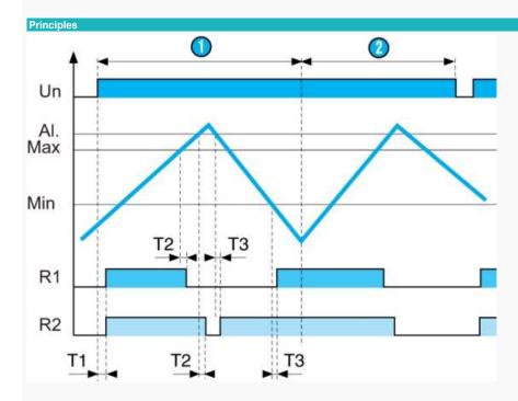
On power-up, the level in the tank is low, relays R1 and R2 are energised and the pump is ON: filling starts, the LED for relay R1 is lit. When the level reaches the Max probe, relay R1 de-energises and the pump is OFF: filling stops, the relay LED goes off. If, in the event of a fault, the level continues to rise and reaches proble Al., relay R2 de-energises and the alarm is triggered: the LED for relay R2 is lit.
