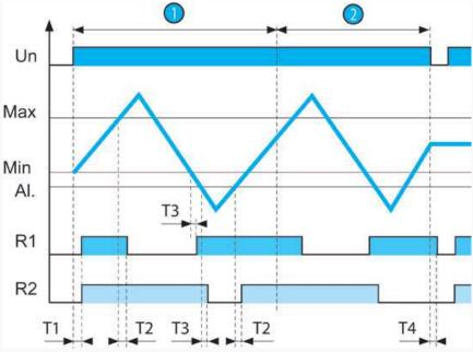
On power-up, probe Al. is submerged, relays R1 and R2 are energised and the pump is ON: filling starts, the LED for relay R1 is lit. When the level reaches the Max probe, relay R1 de-energises and the pump is OFF: filling stops, the LED for relay R1 goes off. Relay R1 re-energises, when the Min probe emerges. In the event of a fault (level continues to fall) probe Al. emerges, relay R2 deenergises an the alarm is triggered: the LED for relay R2 is lit.
