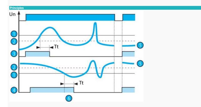
If "with memory" mode has been selected, the relay opens and stays in this position when threshold crossing is detected. The power supply must be disconnected to reset the product.
