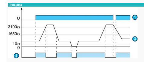
The relay is reset either using the RESET pushbutton on the front face or by opening the external contact S2 (remote reset), or by cutting the auxiliary power supply (terminals A1 - A2). If the auxiliary power is cut for a period of time greater than the reset time (500 ms), the relay is reactivated if the proble detects a normal temperature when the power supply voltage is restored.
