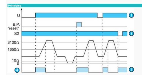
The relay is reset either using the RESET pushbutton on the front face or by opening the external contact S2 (remote reset), or by cutting the auxiliary power supply (terminals A1 - A2). If the auxiliary power is cut for a period of time greater than the reset time (500 ms), the relay is reactivated if the proble detects a normal temperature when the power supply voltage is restored.
