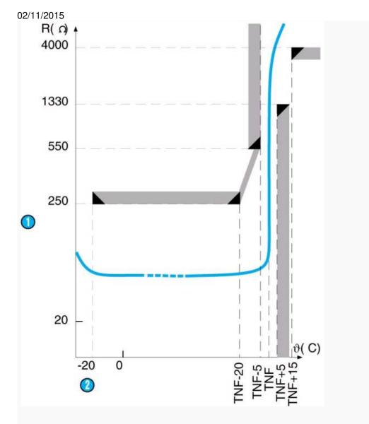
The relay is reset either using the RESET pushbutton on the front face or by opening the external contact S2 (remote reset), or by cutting the auxiliary power supply (terminals A1 - A2). If the auxiliary power is cut for a period of time greater than the reset time (500 ms), the relay is reactivated if the proble detects a normal temperature when the power supply voltage is restored.
