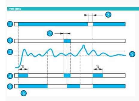
When the HSV has been configured in "memory" mode, if overspeed is detected, the output relay stays in the rest state ("alarm") irrespective of any subsequent change in the speed of the process. It will not be able to revert to ("normal") operating state until contact S2 closes (50 ms minimum). If, when S2 reopens, the speed is too high, the relay reverts to the rest latched state ("alarm").
