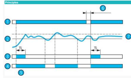
After the end of the inhibit delay on starting, "Ti", as soon as the measured speed drops below the threshold value, the output relay changes state, from operating point to rest position ("alarm" operational state, 11-14 open and 11-12 closed).
