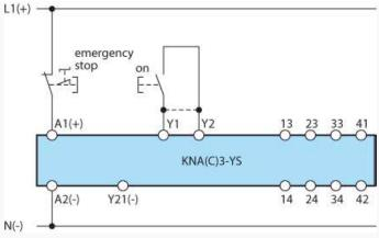
For automatic restart, terminals Y1 - Y2 must be linked. No ON-pushbutton necessary
