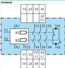
A1 (+): + / L A2: - / N Y1, Y2: Validation Input Y21 (-): Measure Output (-) of secondary used for example in IT networks for insulation control 13, 14, 23, 24, 33, 34: Safety circuit outputs (forcibly guided NO contacts) 41, 42: Monitoring output (forcibly guided NC contact)
