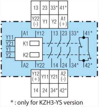
A1 (+):+/LA2:-/NY1, Y2: Feedback circuit input Y11, Y12, Y21, Y22: Control inputs (push buttons) 13, 14, 23, 24, (33, 34) \*: Safety circtui outputs (forcibly guided NO contacts) (41, 42) \*: Monitoring output (forcibly guided NC contact) \*: only for KZH3-YS version
