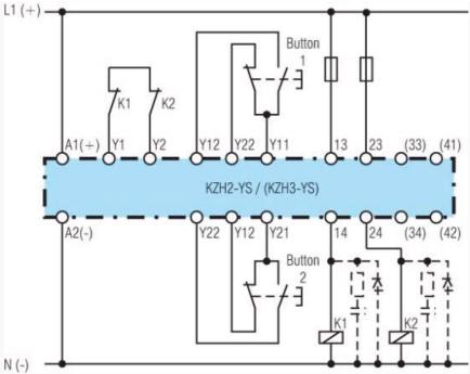
When switching inductive loads, spark absorbers are recommended
