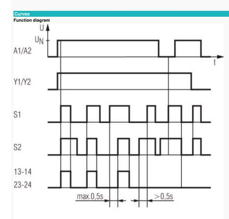
"S1, S2 activated" means, NC open and NO closed
