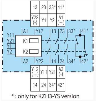
A1 (+) : + / L A2 : - / N Y1, Y2 : Feedback circuit input Y11, Y12, Y21, Y22 : Control inputs (push buttons) 13, 14, 23, 24, (33, 34) \* : Safety circui outputs (forcibly guided NO contacts) (41, 42) \* : Monitoring output (forcibly guided NC contact) \* : only for KZH3-YS version
