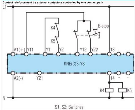
S1 : no cross fault detection S2 : automatic start
