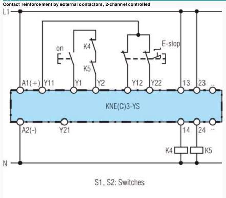
For currents > 8 A, the output contacts can be reinforced by external contactors. Functioning of the external contactors is monitored by looping the NC contacts into the start circuit (Y1-Y2)
