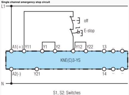
This circuit does not have any redundancy in the emergency-stop control circuit. S1: no cross fault detection S2: automatic start
