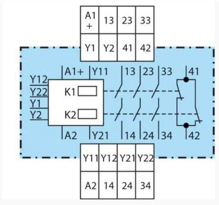
A1 (+):+/LA2:-/NY1, Y2: Validation Input Y11, Y21, Y12, Y22: Control Inputs 13, 14, 23, 24, 33, 34: Safety circuit outputs (forcibly guided NO contacts) 41, 42: Monitoring output (forcibly guided NC contact)
