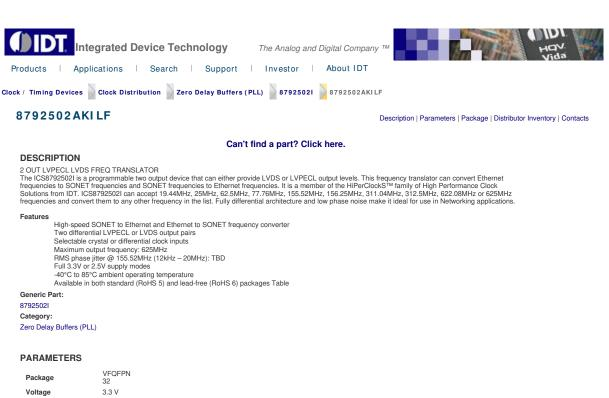
Temperature Speed (19.44 ÷ 25) \* M/N Divide Value Input Style Xtal Max. Input Frequency 627.9355 Min. Input Frequency 19.3466 No. of Outputs 2 **Output Frequency** 625 LVPECL
