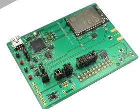
The SN8200 EVK+ facilitates evaluation of and software development around the SN8200 Wi-Fi Network Controller Module. Major enhancements from the previous SN8200 EVK include:
