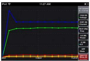
The Smartplug ADK works with the GainSpan Home Energy Management System (HEMS) ADK, which can be used to control multiple smartplugs and thermostats on the home network. The HEMS app allows selection and control of multiple devices, either one-at-a-time or all-together. Once device is selected, the app allows load on/off control as well as a graphical display of the power measurements.
