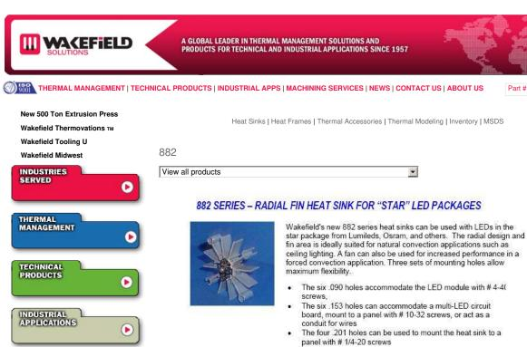
Height "A" Forced Convection Standard Natural Convection Weight Thermal resistance @200LFM P/N in (mm) Temp rise over ambient lbs (grams) 882-50AB 0.50 (12.7) 60 °C @ 9 W 4.33 °C/W 0.073 (34) 882-100AB 1.00 (25.4) 48 °C @ 9 W 2.88 °C/W 0.146 (67) 882-200AB 2.00 (50.8) 36 °C @ 9 W 1.89 °C/W 0.293 (133) 1.55 °C/W 882-300AB 3.00 (76.2) 28 °C @ 9 W 0.439 (199)
