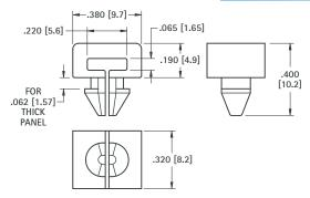
Recommended Mtg. Hole .187 (4.8) diameter.
