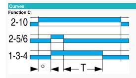
Function C Timing after impulse (delay off) 02/11/2015 www.crouzet.com
