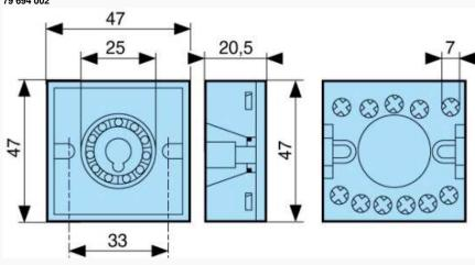
Dimensions (mm) 8-pin or 11-pin solder-connected plug 25 622 076 - 25 622 301
