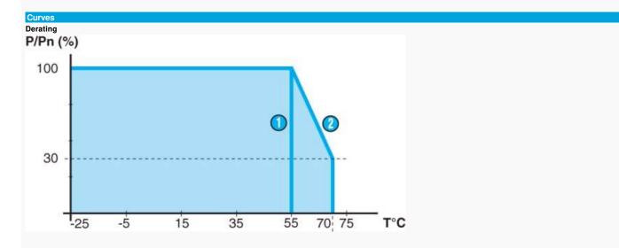
The ambient operating temperature of the Millenium power supplies is 55 °C. Above this, a derating is needed upto a maximum operating temperature of 70 °C. The chart below shows the power (compared to the nominal power) that can be permanently supplied by the power supply, depending on the operating temperature.
