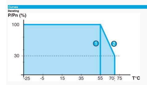
The ambient operating temperature of the Millenium power supplies is 55 °C. Above this, a derating is needed upto a maximum operating temperature of 70 °C. The chart below shows the power (compared to the nominal power) that can be permanently supplied by the power supply, depending on the operating temperature.
