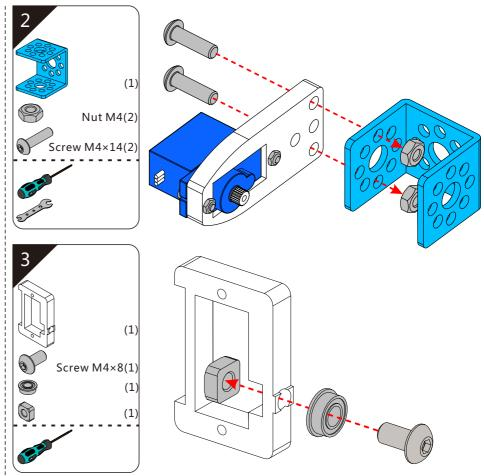
※为了避免用力过大使零件断裂,请使用小力拧螺丝。 ※Gently tighten the screws to avoid any fracture caused by too much fouce.
